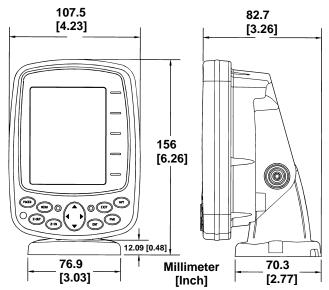
Front view (left) and side view (right) showing dimensions of the Cuda 250 when mounted on quick release bracket.
